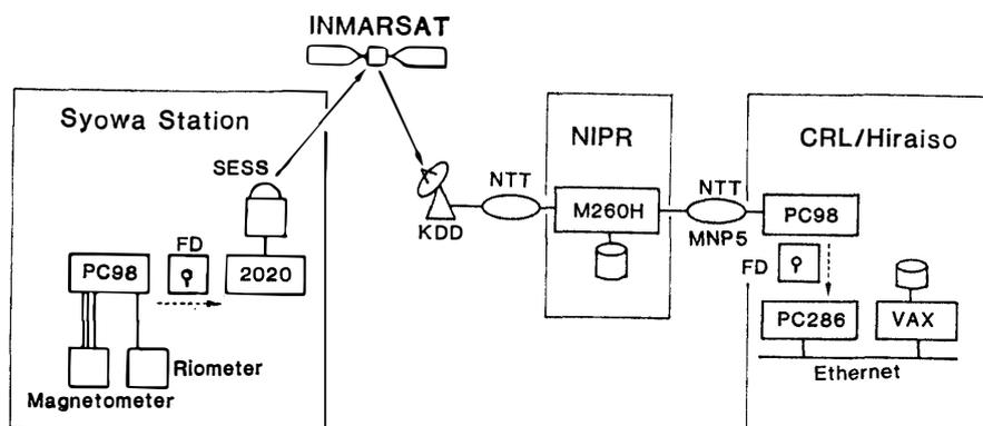
Fig. 1. Outline of the acquisition and transfer system for observational data of Syowa Station using INMARSAT link. The data include the  $H, D, Z$  components of geomagnetic field and the cosmic noise absorptions.
