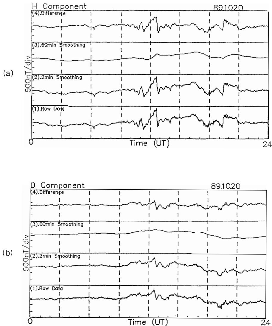
Fig. 2. (a) Horizontal and (b) D components of the geomagnetic field at Syowa Station on October 20, 1989, illustration of the method used in computing *J*-indices. The lower curves, (1) in the figures indicate the raw (unsmoothed) data. The middle two curves, (2) and (3) indicate smoothed data with time constants of 2 min and 60 min, respectively. The top curves, (4) is the difference between (2) and (3).
