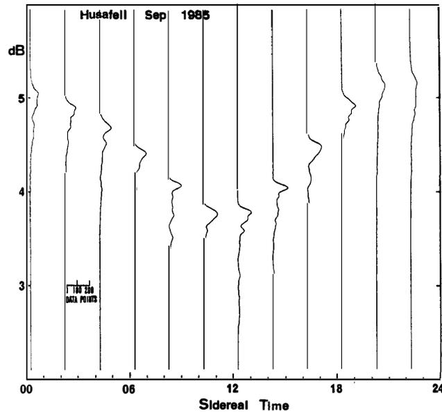
Fig. 4. Examples of actual noise level values at different sidereal times with the corresponding inflection points determined by the program. Each profile shows a measure of the number of data points in a 1/1200 dB interval and a 10 minute bin around the indicated sidereal time (ST).
