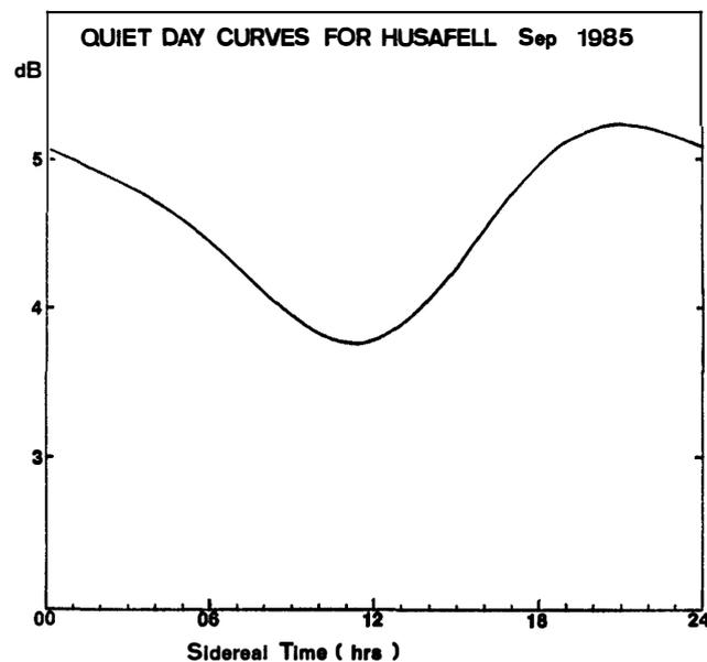
Fig. 5. Quiet day curve computed using the observed dB values for the data set. Fourier analysis was used for data smoothing.
