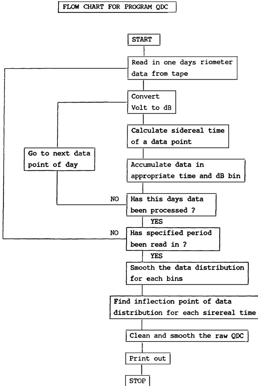
Fig. 2. Flow chart showing the major steps in the Inflection Point Method for obtaining the quiet day curve (QDC) from riometer data.
