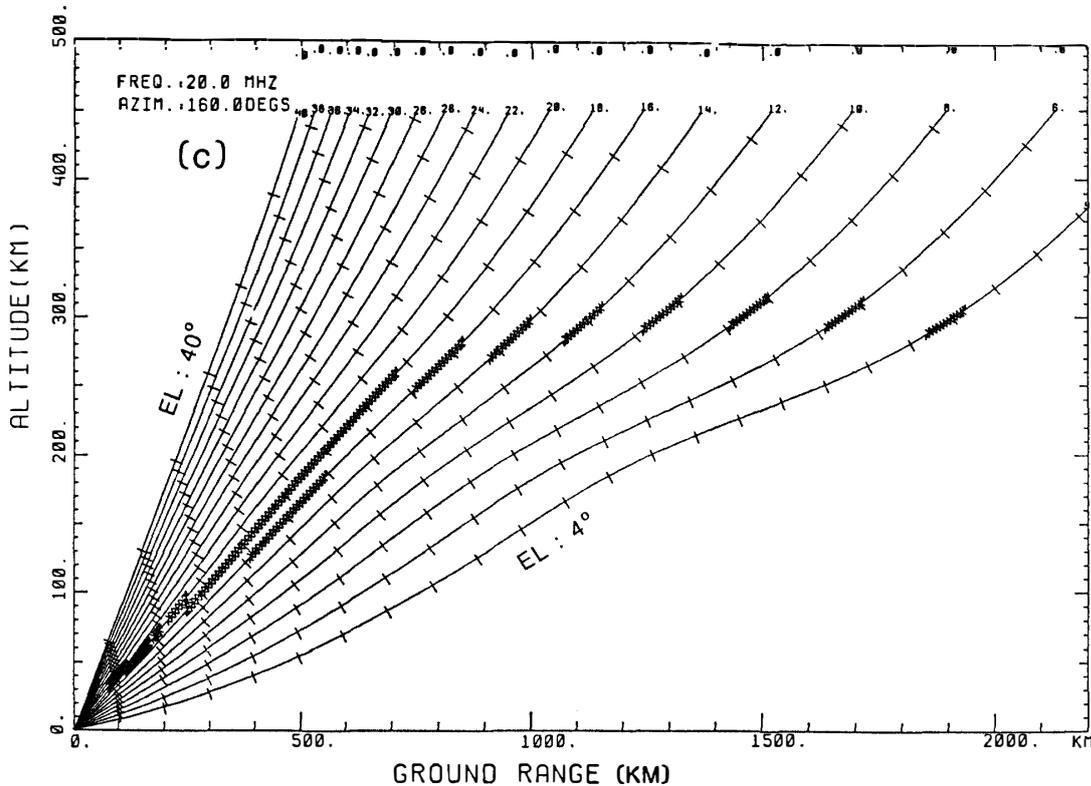
Fig. 1. Ray-tracings for three waves, (a) 10 MHz, (b) 15 MHz and (c) 20 MHz, emitted from Syowa Station with elevation angles of  $4^{\circ}$ – $40^{\circ}$  ( $2^{\circ}$  step) at an azimuth of  $160^{\circ}$ . Positions where ray paths are nearly perpendicular (between  $89^{\circ}$  and  $91^{\circ}$ ) to the geomagnetic field are indicated by the crosses. A Chapman-type ionospheric electron density distribution is assumed for the calculations.
