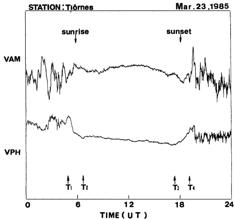
Fig. 4a. Diurnal variation in the phase and amplitude of the 12.1 kHz band Omega signal observed at Tjörnes on March 23, 1985. The times of sunrise and sunset at Tjörnes are also indicated in this figure.
