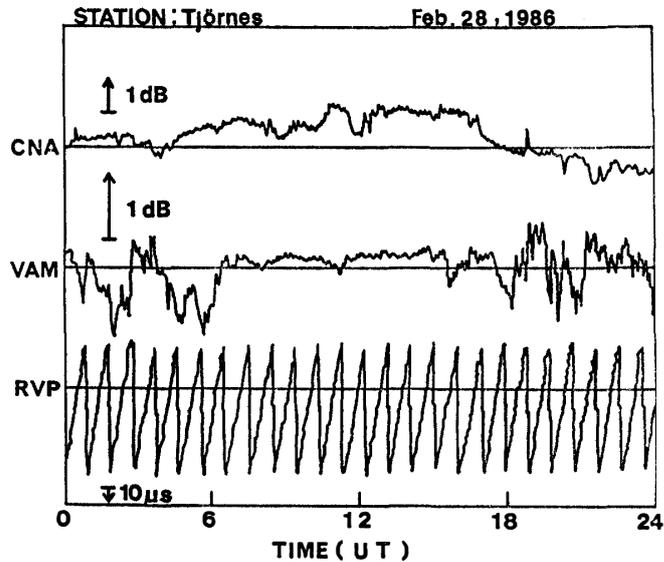
Fig. 2. Diurnal variations in the riometer and VLF signals at Tjörnes in Iceland. CNA: cosmic noise absorption. VAM: Amplitude of VLF omega signals. RVP: Raw data plot of raw VLF phase change.
