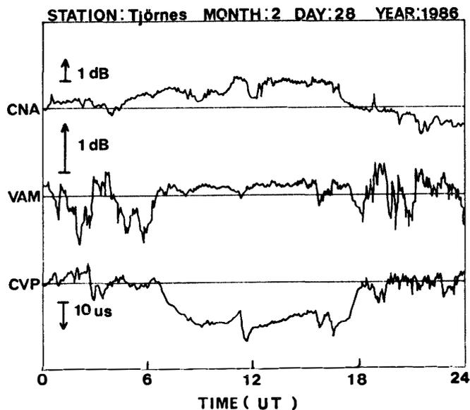
Fig. 3. Diurnal variation in the riometer and VLF signals at Tjörnes in Iceland. CVP: Corrected data plot of VLF phase change.
