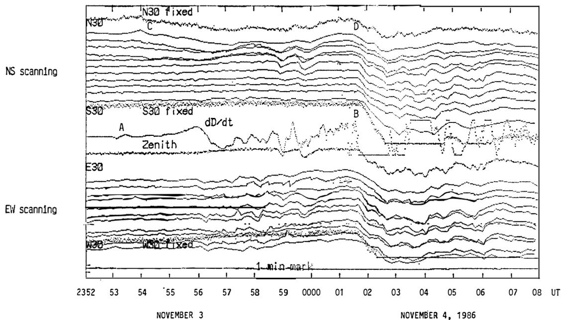
Fig. 2. Cosmic noise absorptions associated with a storm sudden commencement (denoted by C in the figure) and substorm (D), observed by the north-south and east-west scanning beams. The onsets of the SSC and substorm are indicated with A and B by the curve of ULF D-component ( $dD/dt$ ).
