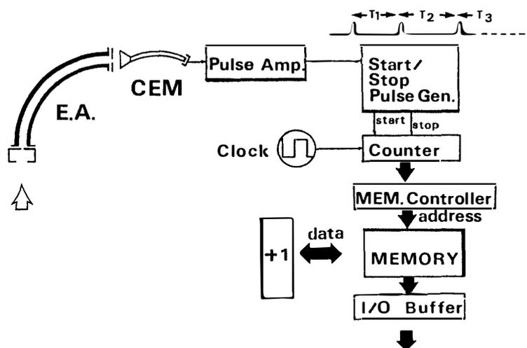
Fig. 1. Block diagram of the pulse separation method.
