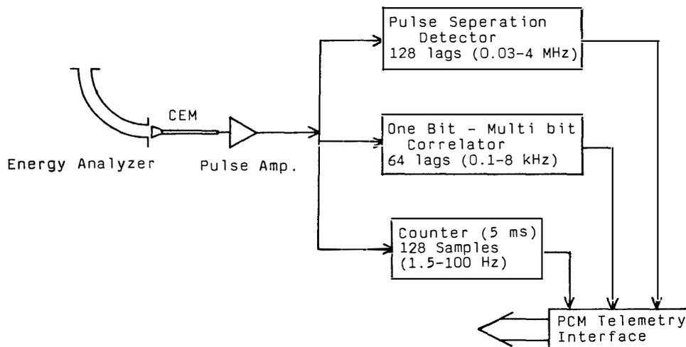
Fig. 3. Functional block diagram of the rocket-borne particle flux modulation detector package (PFMD).
