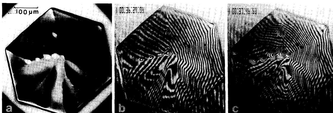
Fig. 1. (0001) face of an ice crystal evaporating in air of  $5.3 \times 10\ \text{Pa}$  at  $-15^\circ\text{C}$  and just below ice saturation. (a) Differential interference image. (b, c) Interference fringes of equal thickness. (a) 0, (b) 45, (c) 79 s.
