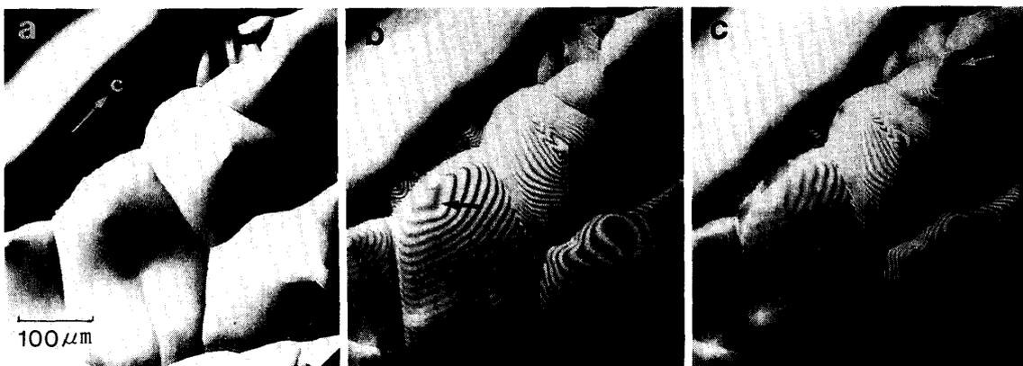
Fig. 3.  $(10\bar{1}0)$  face of an ice crystal evaporating in air of  $5.0 \times 10\ P_a$  at  $-15^\circ\text{C}$  and with increasing subsaturation at the rate of  $0.146\%/s$ . (a) Differential interference image. (b, c) Interference fringes of equal thickness. (a) 0, (b) 23, (c) 40 s.
