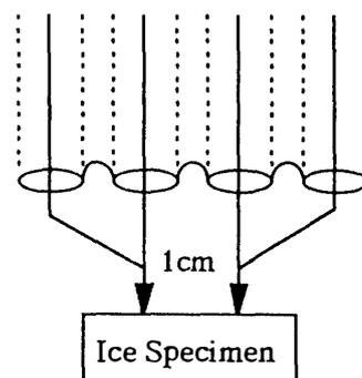
Fig. 2. Diagram of the AC-ECM electrodes. These electrodes form a 4-terminal network. However only two terminals are contacted directly to the ice surface, the other two outer terminals are connected to the inner terminals near the ice surface. The two inner terminals were stainless-steel rods of diameter 3.0 mm. The radius of curvature at the edge of each terminal is 1.5 mm. The distance between the inner terminals is 1 cm.
