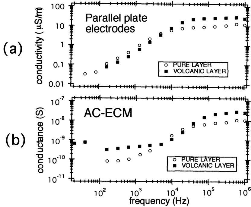
Fig. 5. A schematic representation of the behavior of electrical conduction of Antarctic ice measured with two electrodes; (a) conductivity ( $\mu\text{S/m}$ ) measured with parallel-plate electrodes and (b) the conductance (S) measured by the AC-ECM; at a point in the ice layer containing volcanic ash at a point in the adjacent layer.
