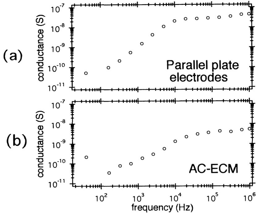
Fig. 4. A schematic representation of the behavior of the conductance of pure ice as a function of frequency near  $-20^{\circ}\text{C}$ . The result in (a) is measured by the AC-ECM technique. The result in (b) is measured with parallel plate electrodes.
