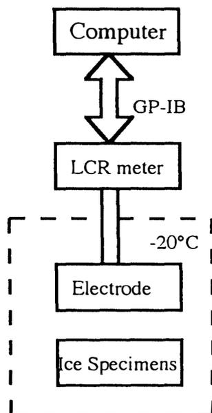
Fig. 1. Schematic diagram of the AC-ECM technique. The system consists of the electrodes and a Precision LCR meter (Hewlett-Packard 4284A). The system was controlled by computer. The experimental temperature was  $-20(\pm 1)^{\circ}\text{C}$ .
