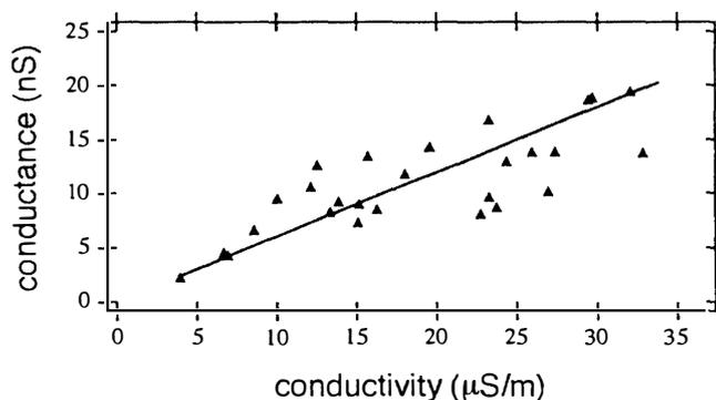
Fig. 7. Relationship between conductivity ( $\mu\text{S/m}$ ) measured by the parallel plate electrode to conductance (nS) measured by the AC-ECM technique.
