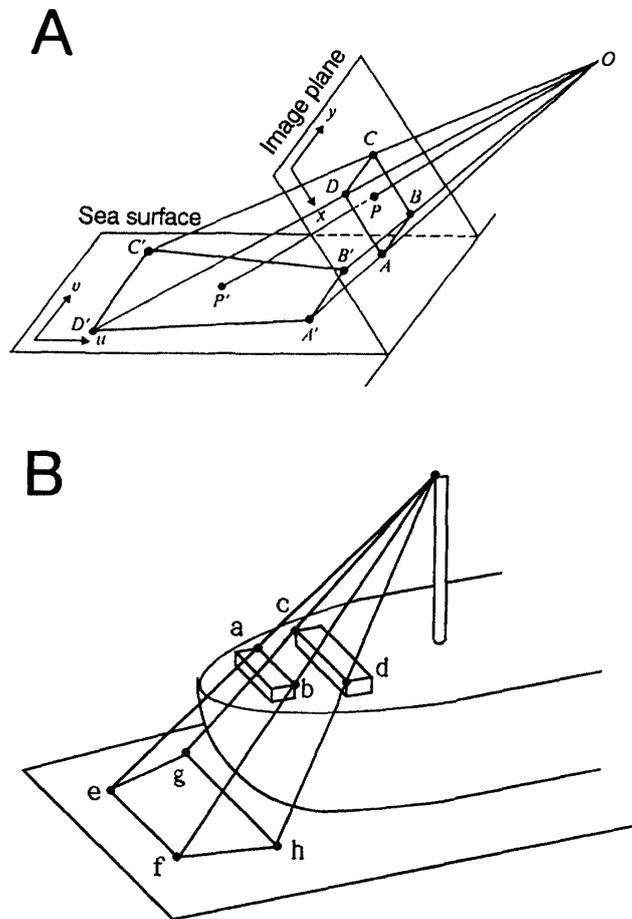
Fig. 2. A: Spatial relation between the sea surface and its perspective projection in the image plane. B: Using known points (a-h), initial coordinates A-D are transformed to A'-D'.
