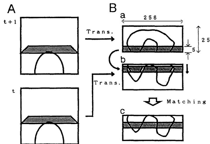
Fig. 3. Schema of template matching. A: Oblique projections at times  $t$  and  $(t+1)$ . B: Orthographic projection transformed from the trapezoidal region shown in A by oblique projection. a: Template pattern. b: Search picture. c: Result of matching at offset location.
