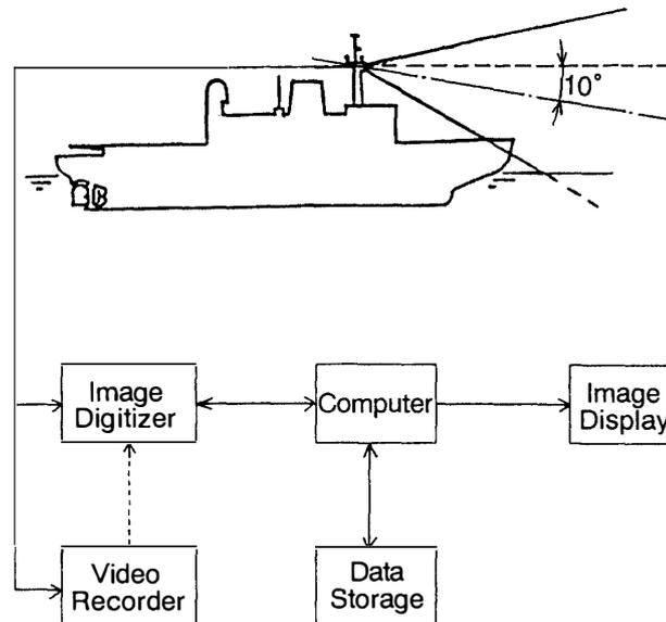
Fig. 1. System configuration for photographing sea ice and analyzing the image. The camera was located at the upper steering house at an angle of  $10^\circ$  downward from the horizon.
