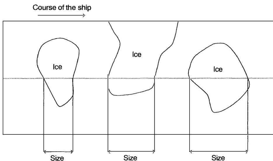
Fig. 4. Method of calculation of floe size distribution.
