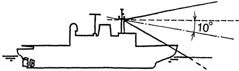
Fig. 1. System configuration for photographing sea ice. The camera was located at the upper steering house with an angle of  $10^\circ$  downward from the horizon.
