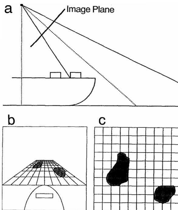
Fig. 2. Schema of geometric transformation. a) Spatial relation between the sea water and its projection in the image plane. b) Oblique projection. c) Orthographic projection transformed from trapezoid region (shown in b) on oblique projection.
