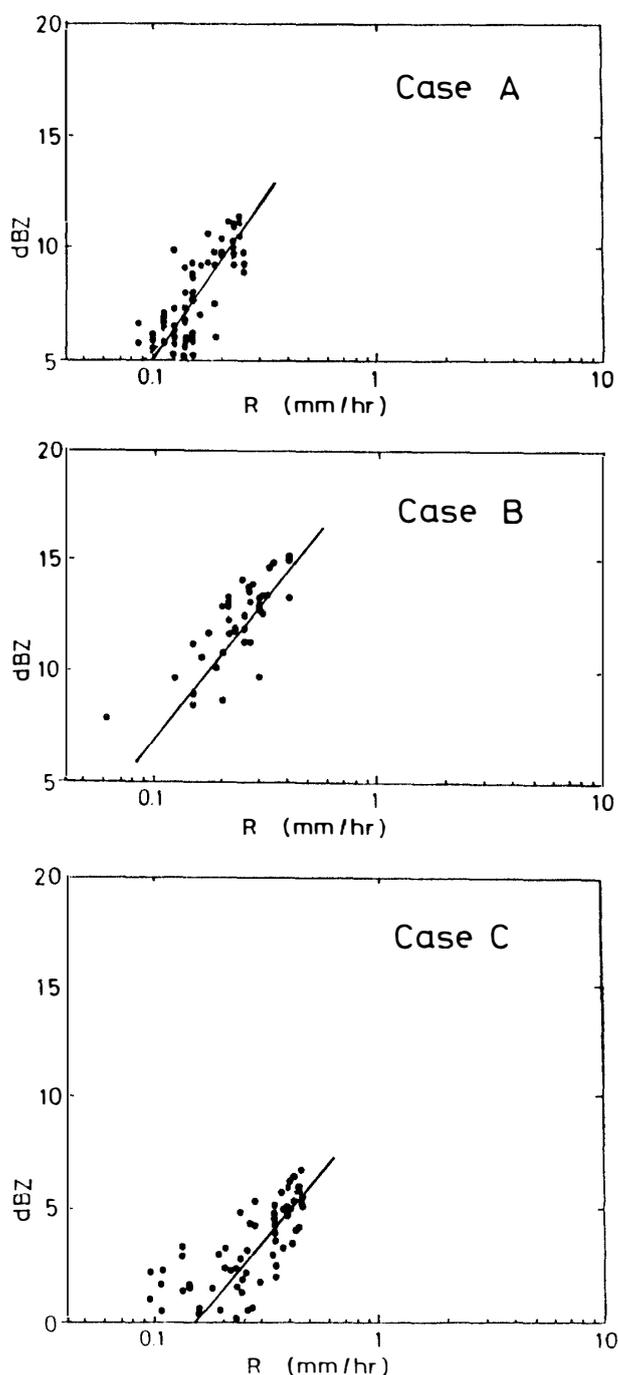
*Fig. 2. The relationship between snowfall rate and radar reflectivity factor observed at Syowa Station (Case A: October 25, 1989, Case B: July 1, 1989, Case C: May 22, 1989).*
