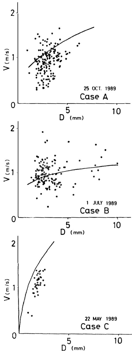
Fig. 1. Fall velocity versus diameter of snow particles at Syowa Station. The lines show the best fit curve for particles by LOCATELLI and HOBBS (1974). A: Aggregates of unrimed side planes assemblages of plates bullets and columns, B: Aggregates of unrimed dendrites and radiating assemblages of dendrites, C: Hexagonal graupels.
