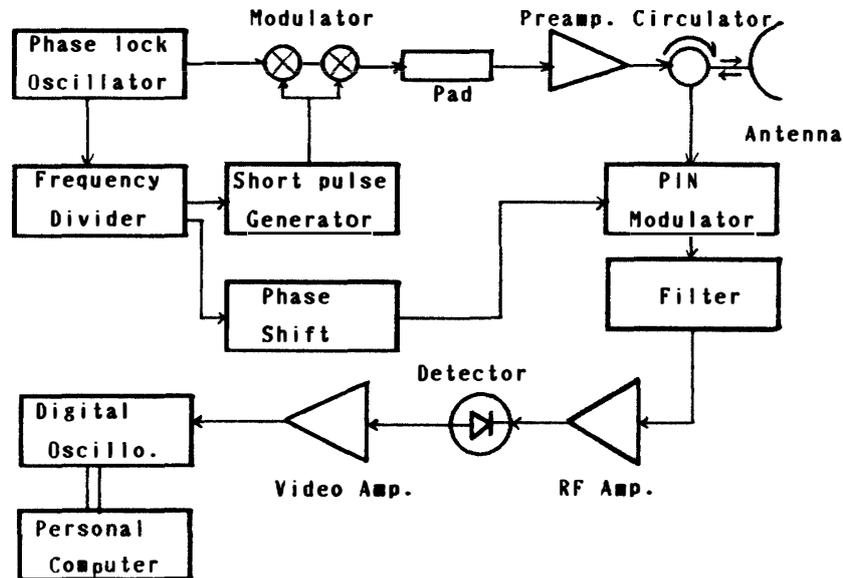
Fig. 2. Block diagram of a C-band radar for hidden crevasse detection with a very short pulse length.
