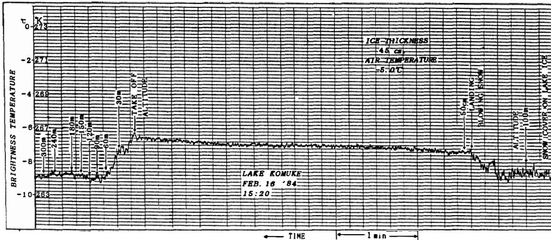
Fig. 5. Brightness temperature for various surface conditions, obtained at Lake Komuke near Mombetsu Airport.
