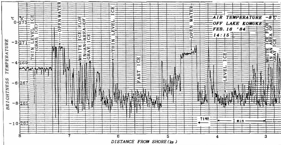
Fig. 2. Brightness temperature distribution observed by the infrared radiometer 3 to 8 km northeast of Mombetsu Airport.
