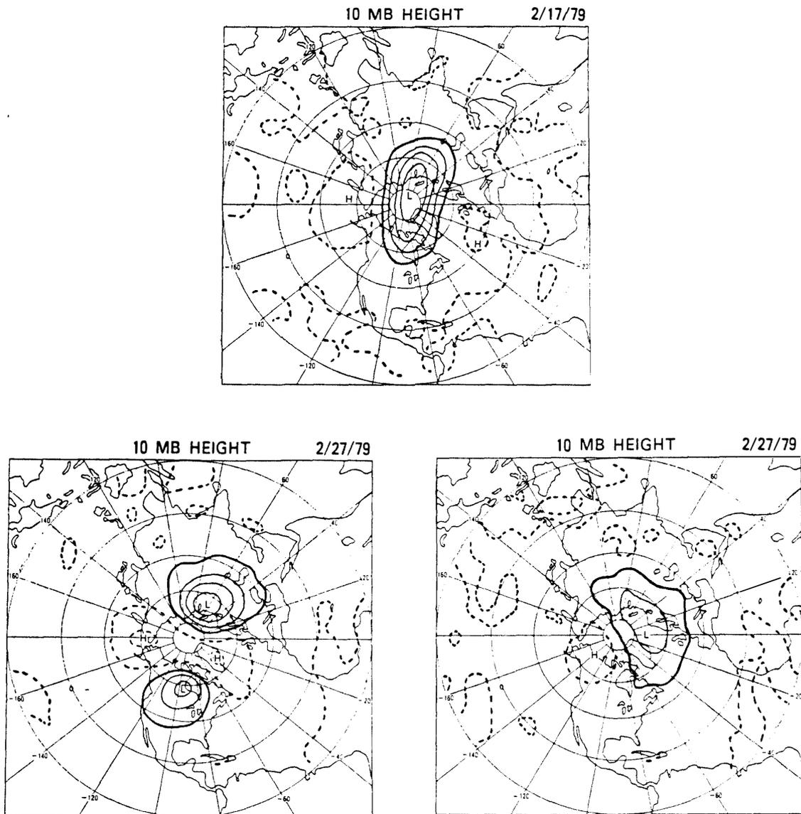
Fig. 3. Height maps of 10 mb in the northern hemisphere forecast by the GMC during a major stratospheric warming. Top panel shows initial condition on 2/17/1979. Bottom panels show the forecast results on 2/27/1979 without (left) and with (right) gravity wave parameterization. Thick solid, 30500 m; thin solid, 30000, 29500, 29000 m; thick dotted, 31000 m; thin dotted, 31500 m.
