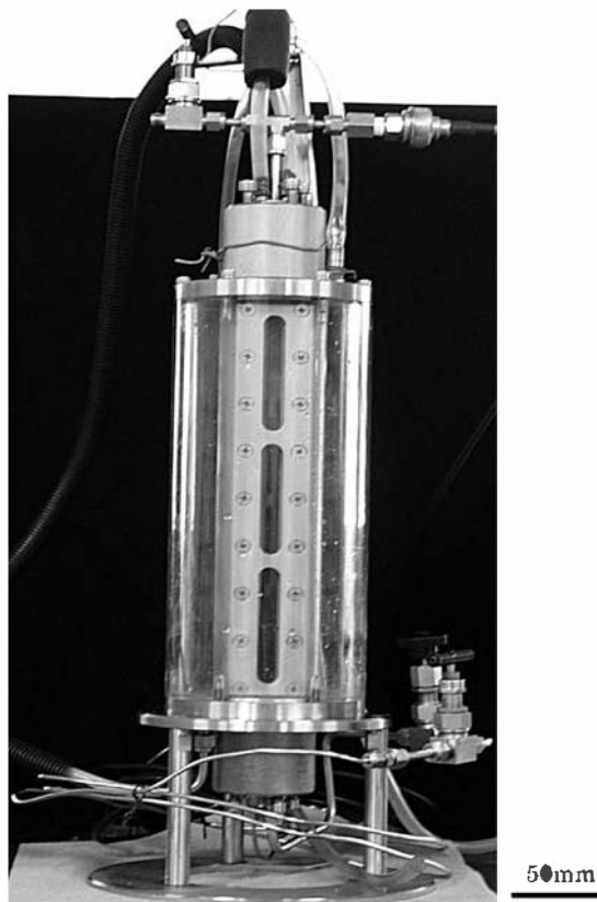
Fig. 1. Pressure cell A for hydrate chimney formation.
