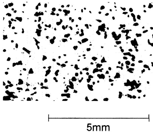
Fig. 3. A section plane of a snow specimen (density is  $200 \text{ kg m}^{-3}$ ) dyed with sudan black B. The contrast of black and white was inverse because the dyed surface slightly melted and reflected the perpendicular lighting to the specimen.
