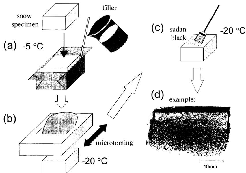
Fig. 1. Preparation of section plane with sudan black B. (a) Pouring the filler into the case and immersing a snow specimen. (b) Shaving the snow specimen after removing the case. (c) Dyeing a section with sudan black B. (d) Example: a section plane visualized with sudan black B. The sample (vertical section) is a layer of partly decomposed precipitation particles sandwiched between layers of rounded grains.
