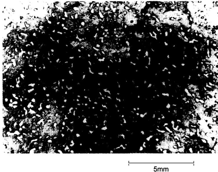
Fig. 4. A section plane of a snow specimen dyed with sudan black B. The filler is dimethyl phthalate.
