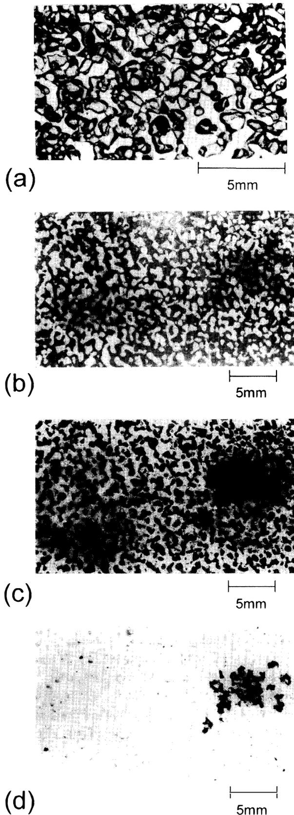
Fig. 2. Thin section and section planes of granular snow (density:  $350 \text{ kg m}^{-3}$ ). Aniline is adopted as a filler. (a) A thin section approx. 0.2 mm in thickness by the aniline method. (b) A section plane dyed with Sudan black B. (c) A section plane obtained by shaving the surface shown in Fig. 2b and dyeing with water blue. The contrast of black and white was inverse to Fig. 2b. (d) A section plane obtained by shaving the surface shown in Fig. 2c.
