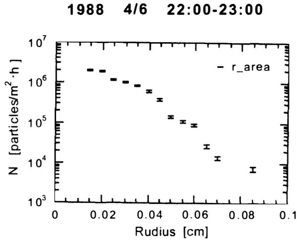
Fig. 5. An example of  $N(r)$  and  $N_+(r)$ : the lower limit bar shows  $N(r\_area)$  and the upper one shows  $N_+(r\_area)$ .
