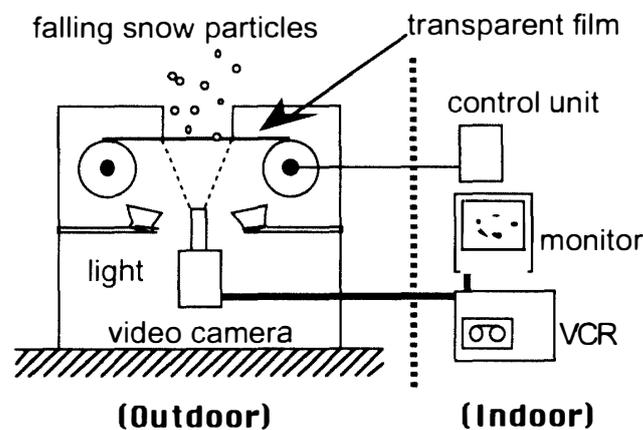
Fig. 1. Configuration of the portable video camera set.
