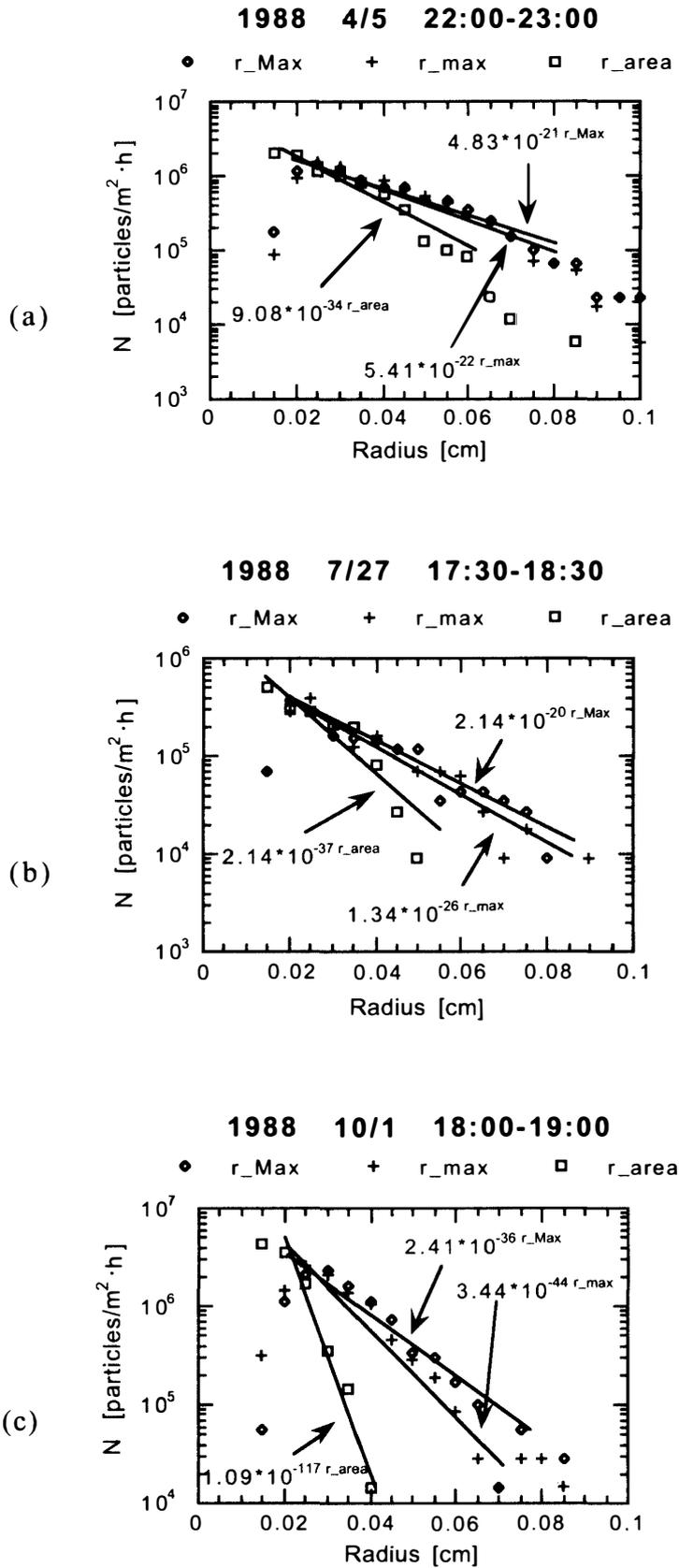
*Fig. 4. Examples of measured snow particle size distributions at Syowa Station, Antarctica in 1988. (a) Tape a: from 2200 LT to 2300 LT on April 5, (b) tape b: from 1730 LT to 1830 LT on July 27, and (c) tape e: from 1800 LT to 1900 LT on October 1.*
