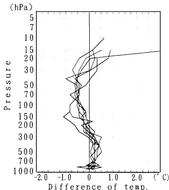
Fig. 1. Vertical profiles of temperature differences  $\Delta T$  (RS2-91 minus RS2-80) at each standard pressure level at Syowa Station, in early September 1996.
