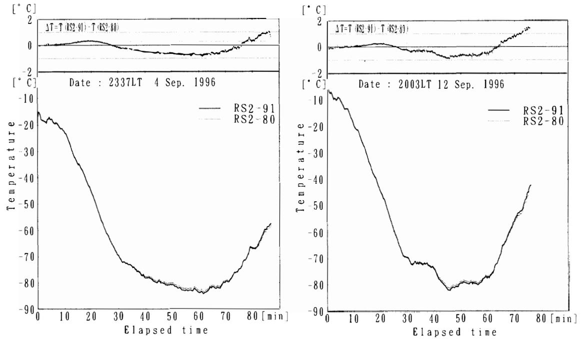
Fig. 2. Temperatures measured by RS2-91 and RS2-80, and the differences  $\Delta T$  as functions of time elapsed from launch.
