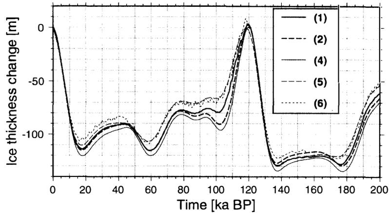
Fig. 5. Ice thickness changes for the different sensitivity experiments at Dome Fuji Station for the last 200 ka of integration in time. (1) standard model run; (2) reduced surface mass balance; (4) without basal melting; (5) with bedrock heat conduction; (6) increased basal sliding.
