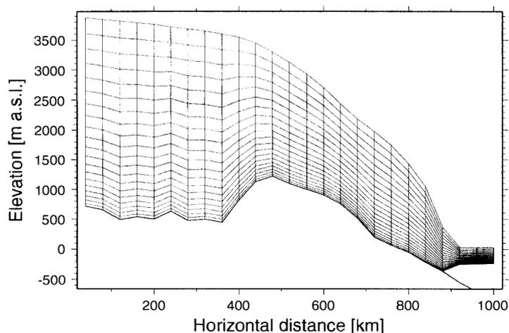
Fig. 2. Model domain on a 40 km grid with 21 layers in the vertical.
