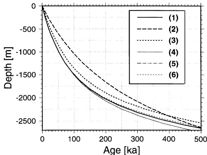
Fig. 3. Age-depth profiles for the different sensitivity experiments at Dome Fuji Station after 1000 ka of integration in time. (1) standard model run; (2) reduced surface mass balance; (3) constant surface mass balance in time; (4) without basal melting; (5) with bedrock heat conduction; (6) increased basal sliding. Curves 1 and 5 overlap.
