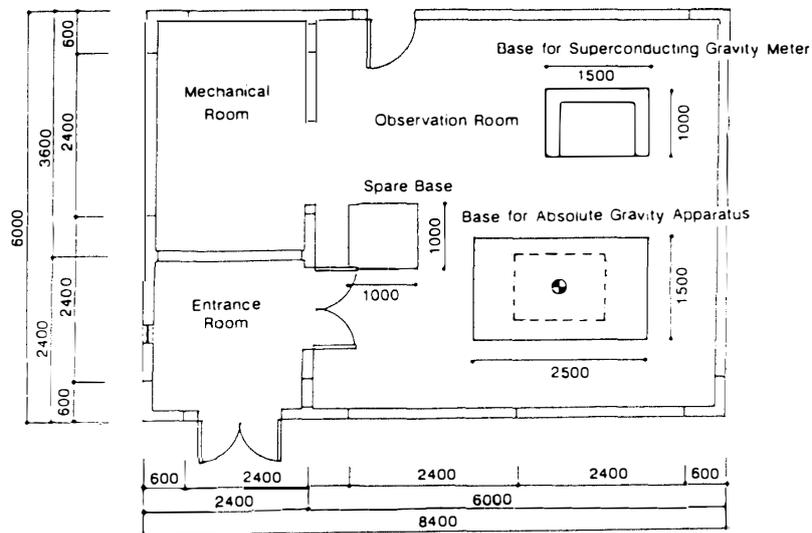
*Fig. 2. Facilities at Syowa Station, and the plain view of the Gravity Observation Hut. There is a concrete pier and base to support the SCG dewar, and another marble base for installing the absolute gravity apparatus.*
