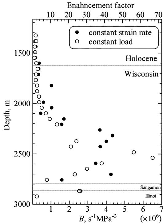
Fig. 3. The result of uniaxial compression tests of the GRIP ice cores, which were prepared from core samples with the stress axis inclined 45° from the core axis.
