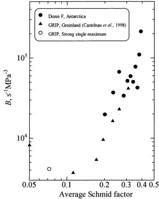
Fig. 4. Flow law parameter versus average Schmid factor of the GRIP and Dome F ice cores.
