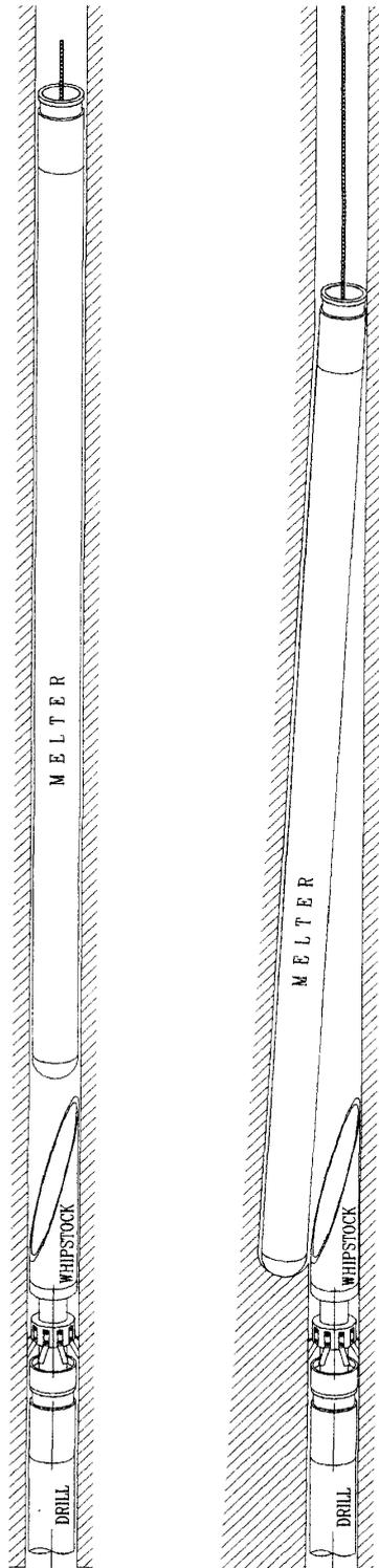
Fig. 4. Application of whipstock for passing object (drill) in the borehole.
