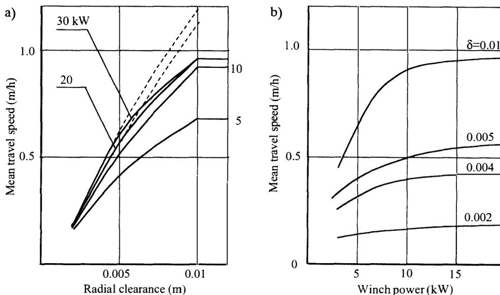
Fig. 1. The mean travel speed versus: a: radial clearance (Solid lines—at  $\nu_{\max}=1$  m/s; Dashed lines—without limitation of hoisting speed); b: winch driving motor power.
