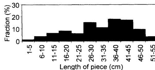
Fig. 7. Histogram of length of ice samples in 1998. The vertical axis denotes the fraction of sum of each fractured ice among certain lengths to the whole core length (14.90 m).
