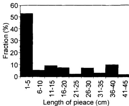
Fig. 5. Histogram of fractured ice length in 1994. The vertical axis denotes the fraction of sum of each fractured ice among certain lengths to the whole core length (23.25 m).
