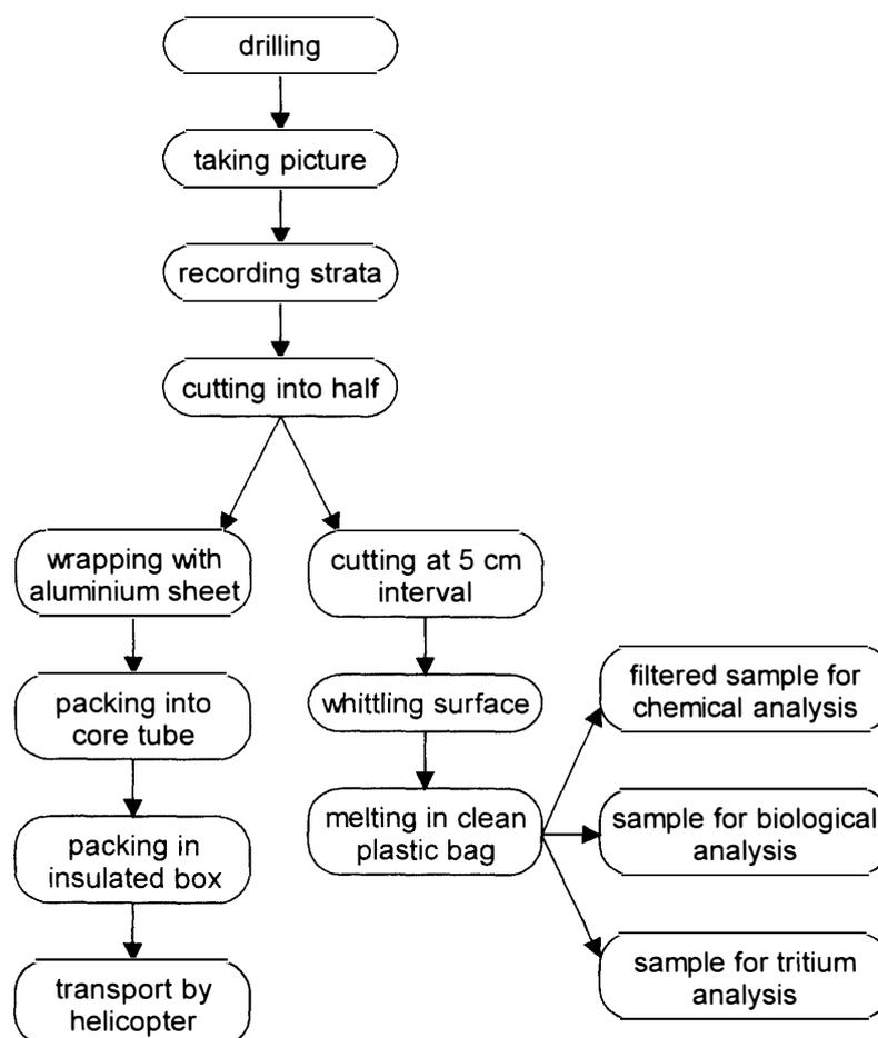
Fig. 8. Schematic flow chart of core process in situ.
