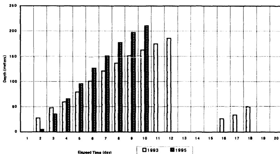
Fig. 2. Daily progress on the drilling depth in 1993 and 1995.
