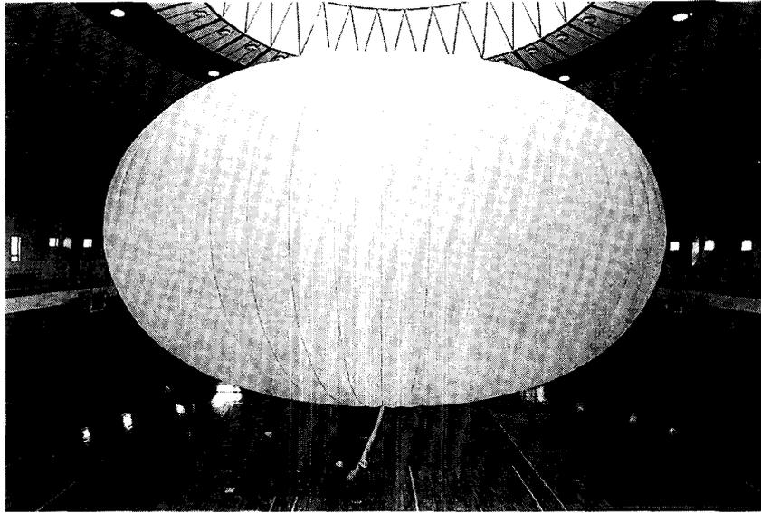
Fig. 6. A 3000 m<sup>3</sup> super-pressure balloon under an indoor inflation test.
