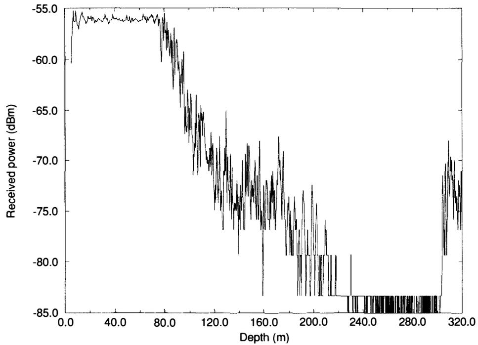
Fig. 4. An example of a radar signal in A-scope form. The location of the data is 1 km south of the summit. The peak around 300 m is from the bottom. The signals in the depth range from 0 to 80 m are saturated. The fine peaks in the range between 80 and 200 m are received from the internal ice.
