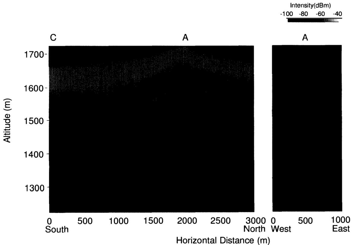
Fig. 3. Preliminary results of ice radar measurement in Z-scope form. The vertical scale is converted from delay time to altitude from sea level.
