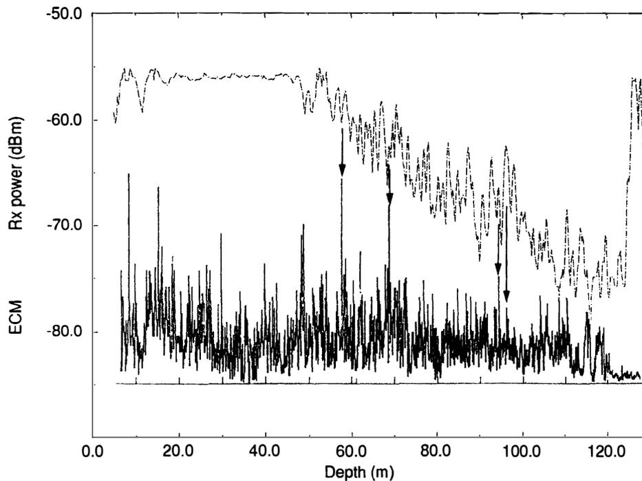
Fig. 6. Comparison between radar echoes observed at site A (upper curve) and the ECM data from the ice core at the same position (lower curve). Some strong peak of ECM data correspond to radar echoes (shown by arrows), but the relation to the intensity is not clear.
