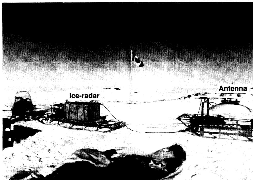
Fig. 2. Observations in progress at the summit of the Agassiz ice cap. Instruments are kept within the heating box on the first sledge after the skidoo, and a 1.2 m diameter parabola antenna for the L-band is mounted on the next sledge.
