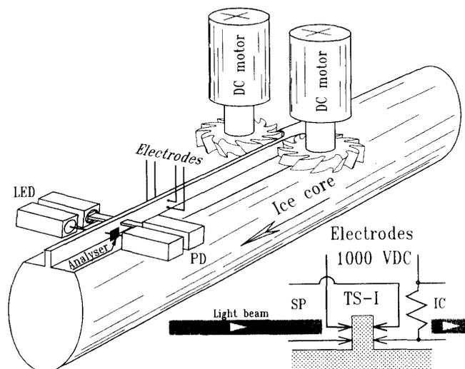
Fig. 1. Schematic of the Ice Core Analytical System: SP—surface potential output, IC—initial current (ECM) output, ED—light-emitting diodes, PD—photo diodes.
