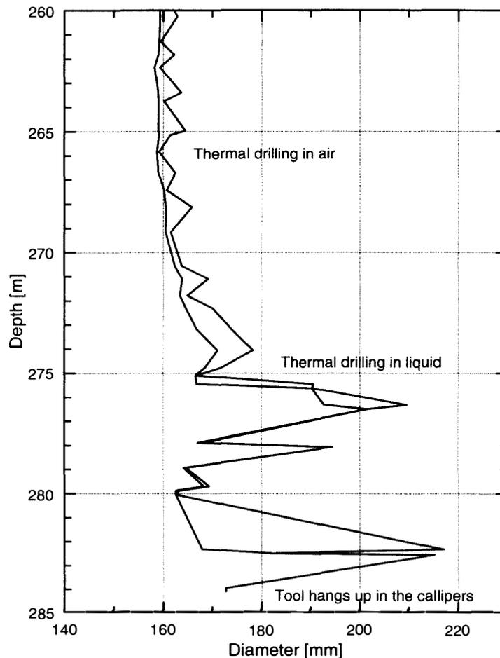
Fig. 5. The lower part of Fig. 4 expanded. It clearly shows the increase in diameter at the core breaks, and the unstable drilling when the operation changed from drilling in a dry hole to thermal drilling in a liquid-filled hole.
