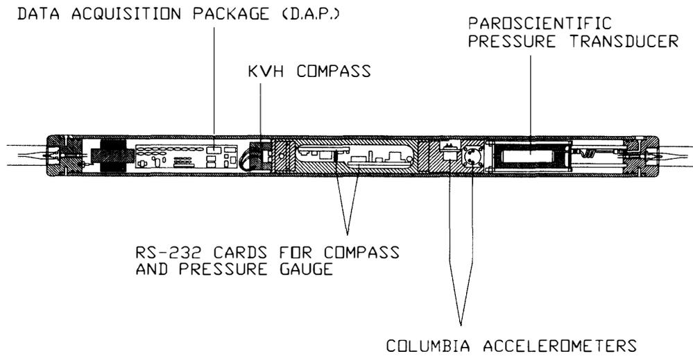
Fig. 1. Short borehole logger.
