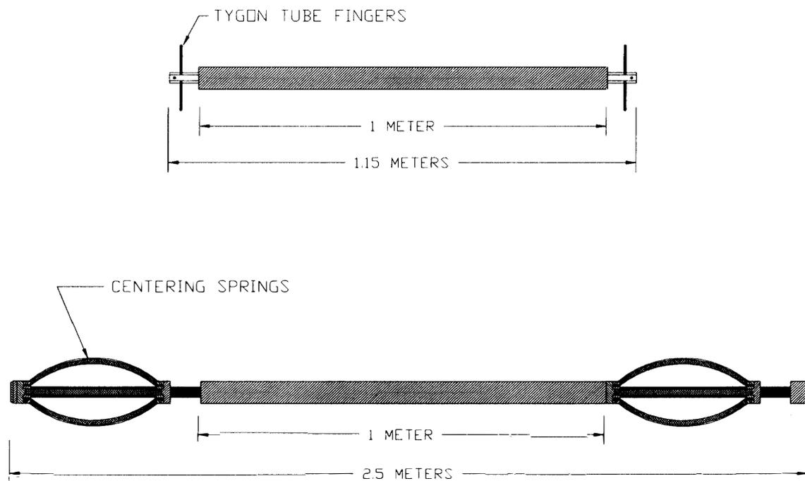
Fig. 4. The short logger with centering springs.
