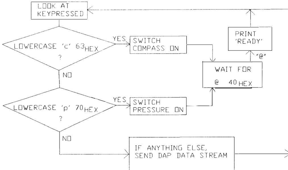
Fig. 3. DAP firmware flow for serial communications MUX control.
