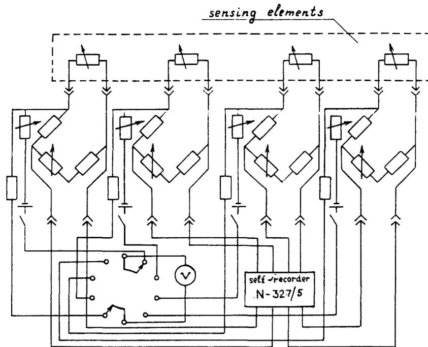
Fig. 2. Electrical diagram of data acquisition system.
