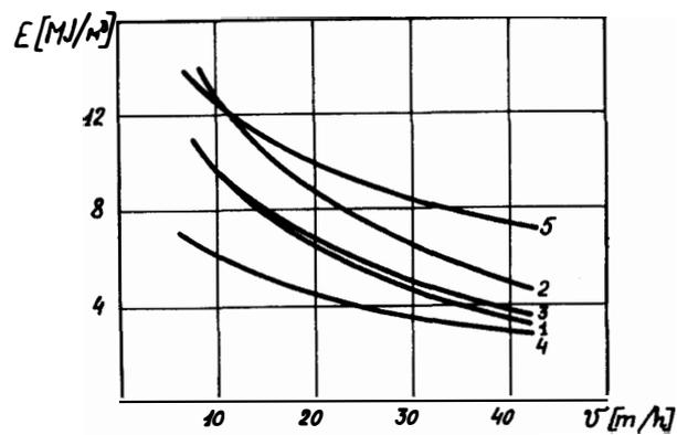
Fig. 8. Specific energy of ice rupture  $E$  versus penetration rate  $v$  for cutters with clearance angle  $5^\circ$  and rake angles  $60^\circ$  (1),  $45^\circ$  (2),  $30^\circ$  (3),  $15^\circ$  (4),  $0^\circ$  (5).
