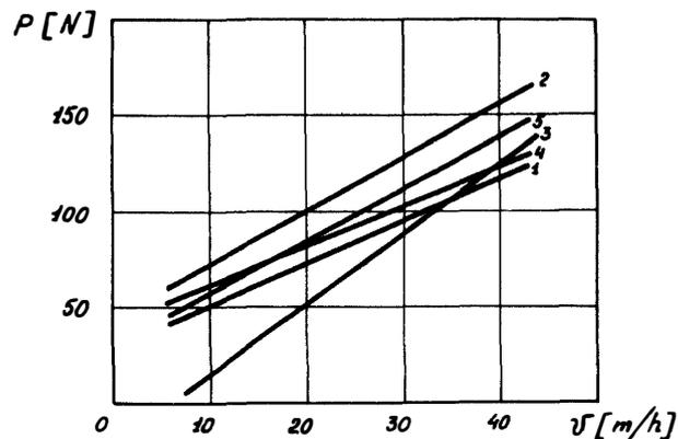
Fig. 5. Drilling pressure  $P$  versus penetration rate  $v$  for cutter with rake angle  $45^\circ$  and clearance angle  $5^\circ$  (1),  $7^\circ$  (2),  $10^\circ$  (3), with rake angle  $15^\circ$  and clearance angle  $5^\circ$  (4), with rake angle  $0^\circ$  and clearance angle  $5^\circ$ .
