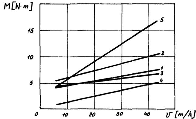
Fig. 4. Torque  $M$  versus penetration rate  $v$  for cutter with clearance angle  $5^\circ$  and rake angles  $60^\circ$  (1),  $45^\circ$  (2),  $30^\circ$  (3),  $15^\circ$  (4),  $0^\circ$  (5).
