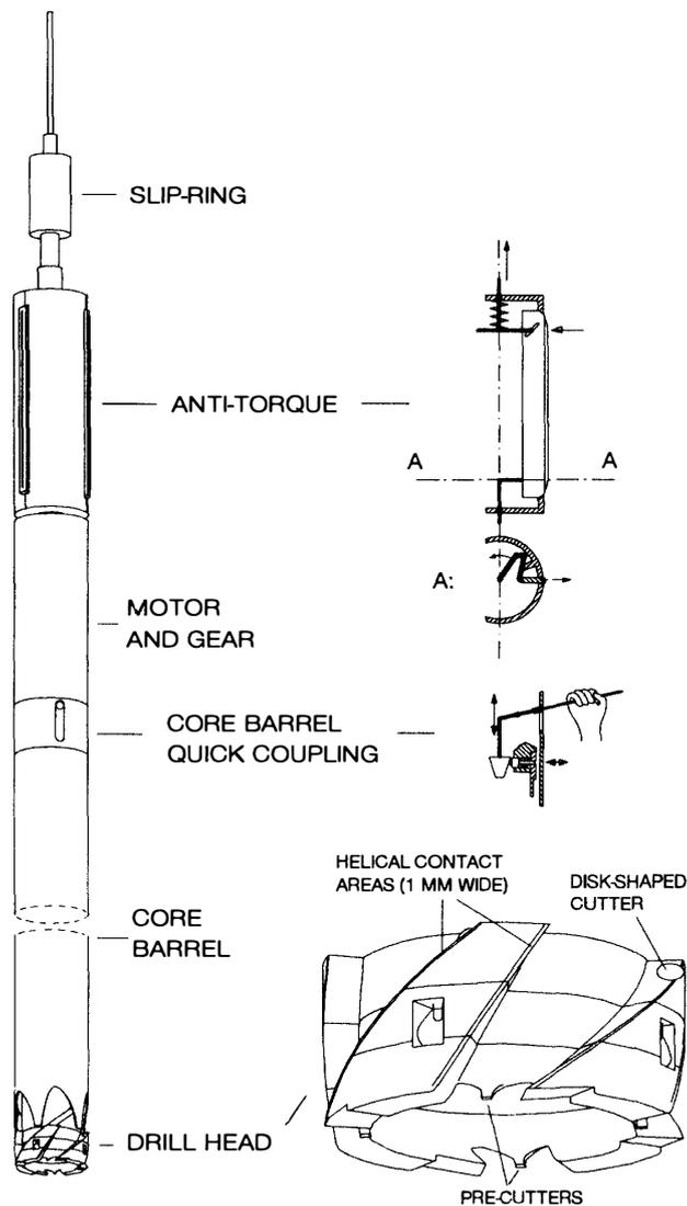
Fig. 2. Drill and drill head. The three skates of the anti-torque section are retracted while hoisting the drill. During drilling the upper part of the skates is activated by a decrease in cable tension and the lower part is forced out by torque.
