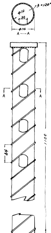
Fig. 2. Structure of the core barrel.
