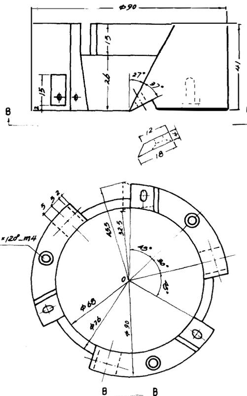
Fig. 3. Structure of the drilling head.
