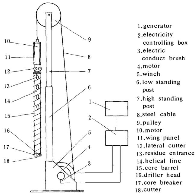
Fig. 1. Schematic of the BZXJ drilling system.
