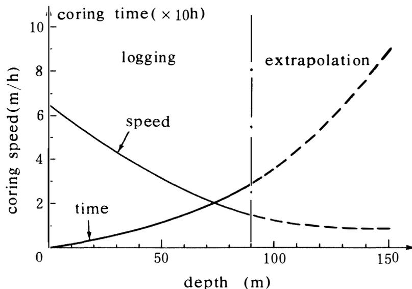
Fig. 4. Penetration performance of the BZXJ drilling system.
