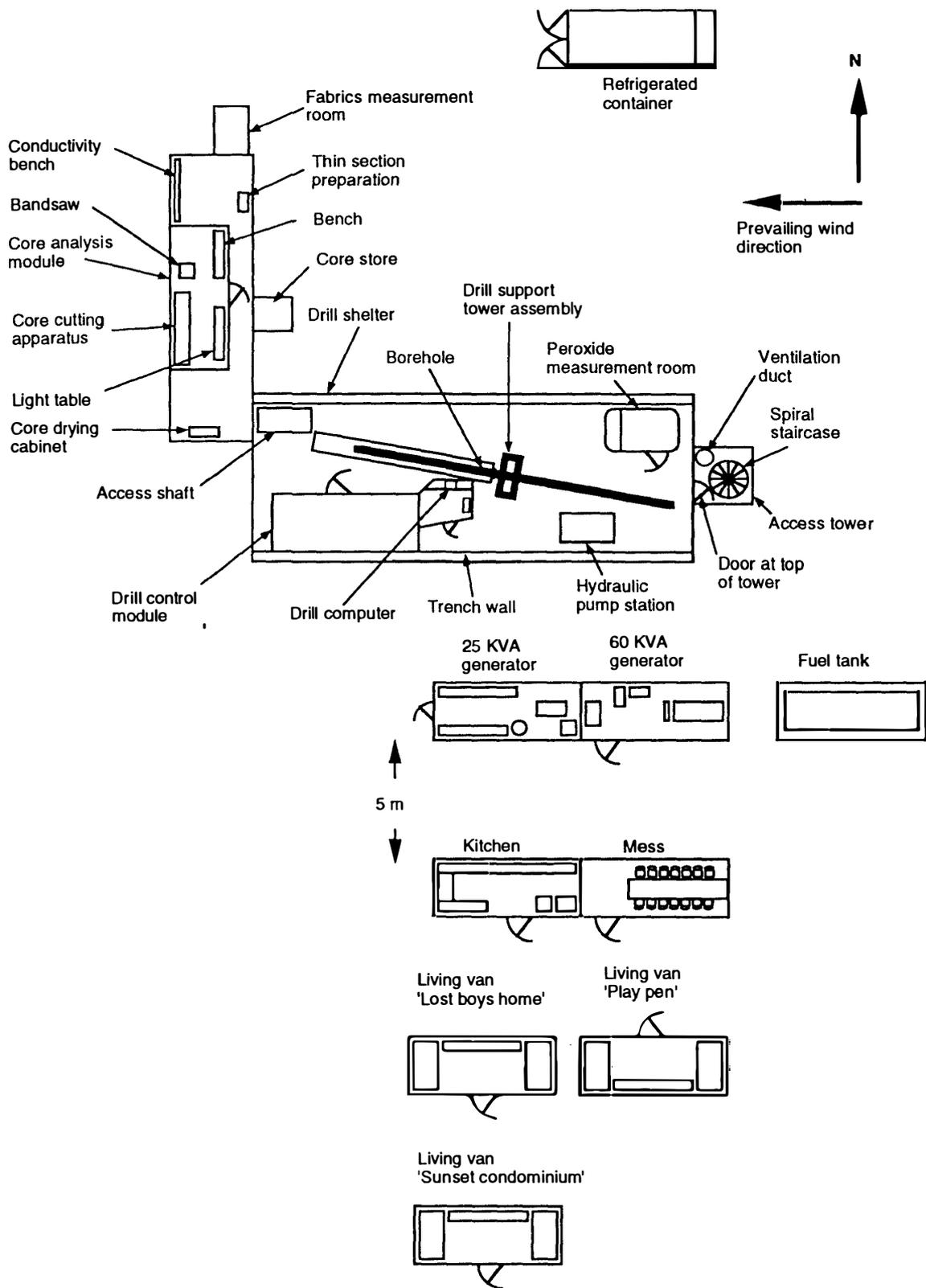
Fig. 3. Dome Summit South (DSS) drilling site-station layout.
