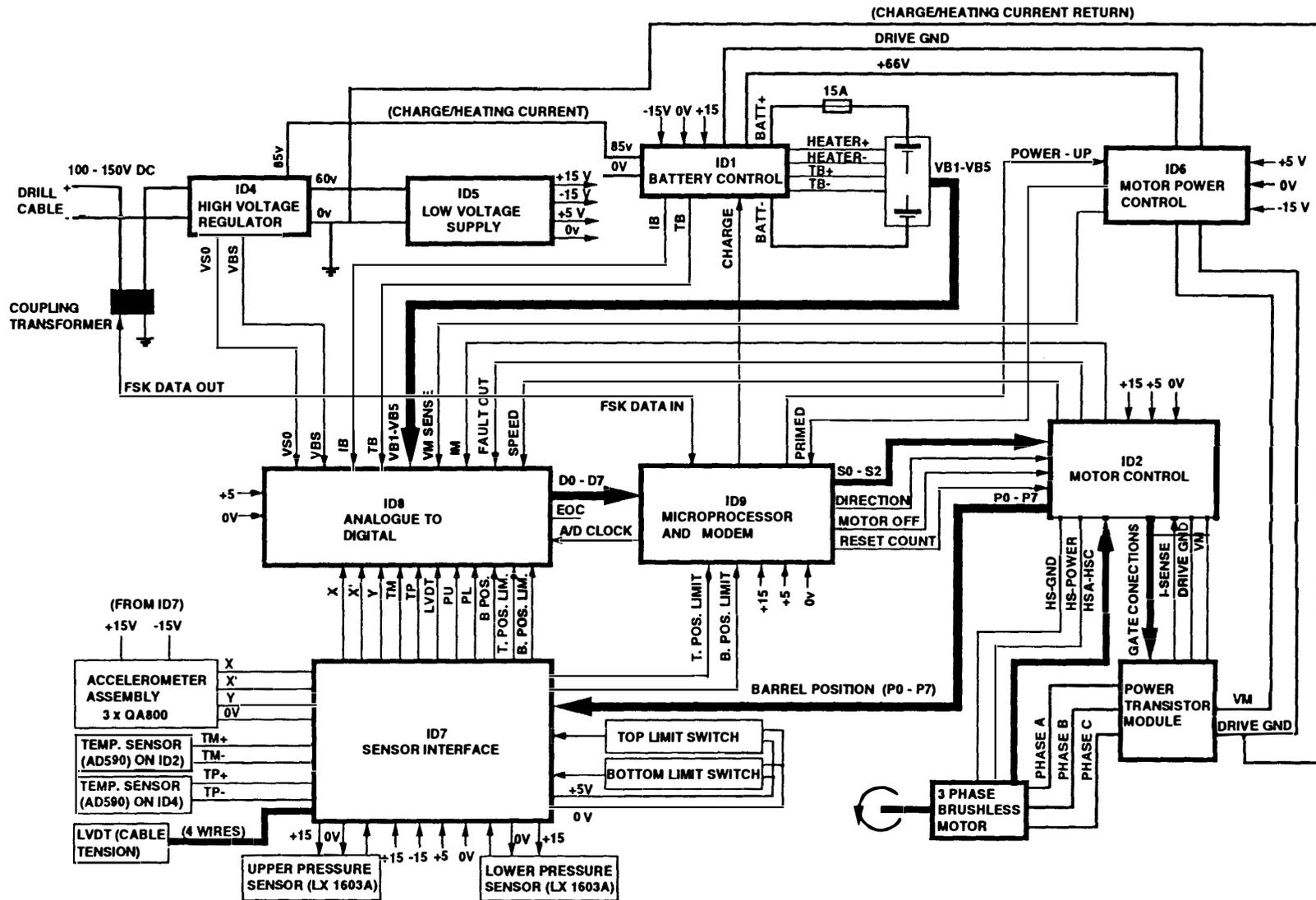
Fig. 2. Ice drill electronics—block diagram.
