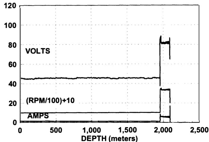
Fig. 5. Drill motor voltage, amps, and rpm (rpm scaled and offset).
