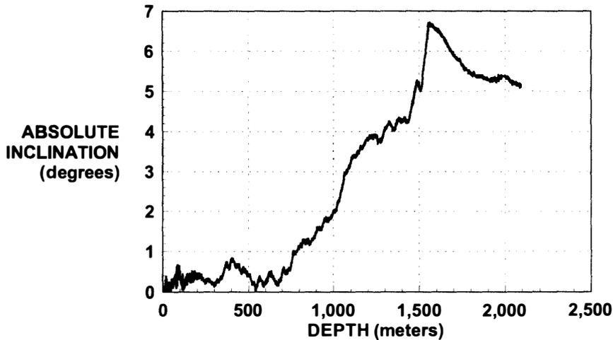
Fig. 8. Calculated borehole inclination versus depth.
