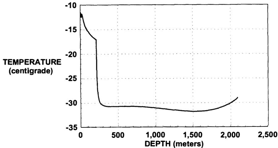
Fig. 4. Temperature in the borehole.
