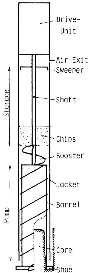
Fig. 1. Schematic diagram of an S-type Archimedean core drill for a dry hole.
