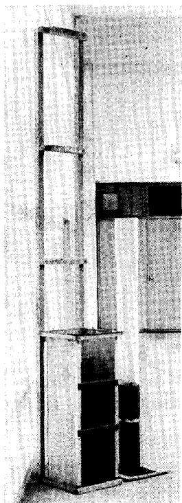
Fig. 3a. The ice box and the hole simulator.
