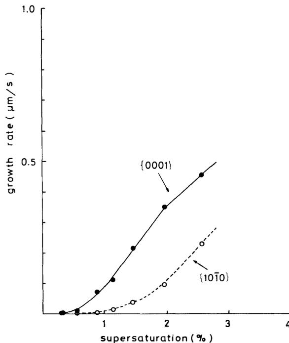
Fig. 4. Supersaturation dependence of the normal growth rates of the  $\{0001\}$  and  $\{10\bar{1}0\}$  faces of a columnar ice crystal grown in air at  $4.0 \times 10$  Pa at  $-30^\circ\text{C}$ .
