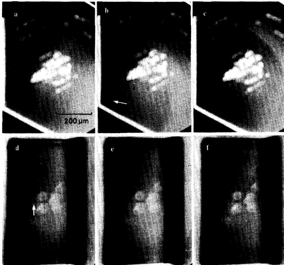
Fig. 5. Surface microtopography of the  $\{0001\}$  and  $\{10\bar{1}0\}$  faces of ice crystals grown in air at  $4.0 \times 10$  Pa at  $-30^\circ\text{C}$ . The upper and lower crystals show the  $\{0001\}$  and  $\{10\bar{1}0\}$  faces, respectively. (a) 0, (b) 5, (c) 10 s; (d) 0, (e) 2, (f) 4 s.
