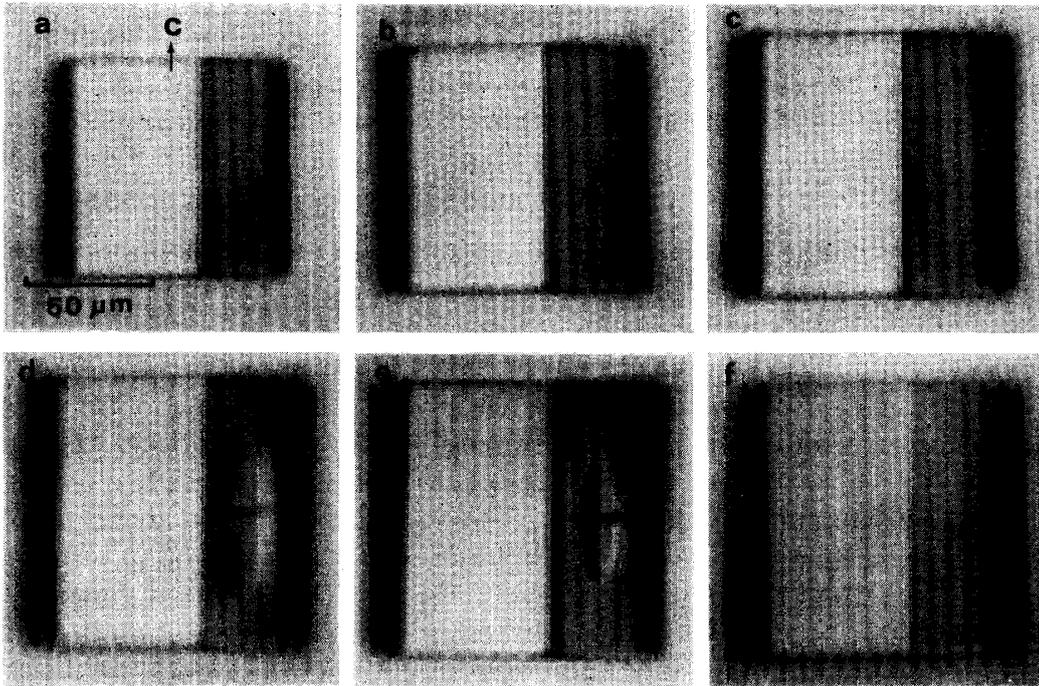
Fig. 2. Ice crystal grown in air at  $1.0 \times 10^5$  Pa at  $-30^\circ\text{C}$  and 0.8% supersaturation, whose size ratio  $c/a$  is close to unity. (a) 0, (b) 44.7, (c) 74.6, (d) 89.6, (e) 96.6, (f) 100 min.
