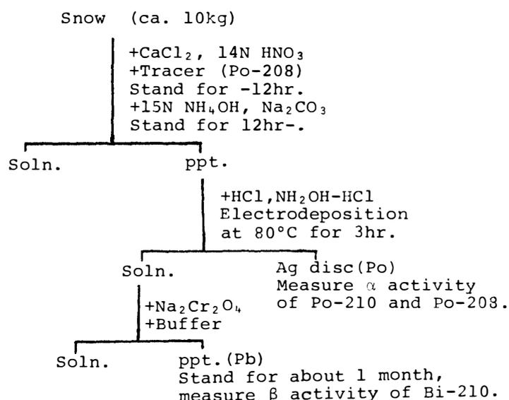
Fig. 2. The procedure for determination of Po-210 and Pb-210.
