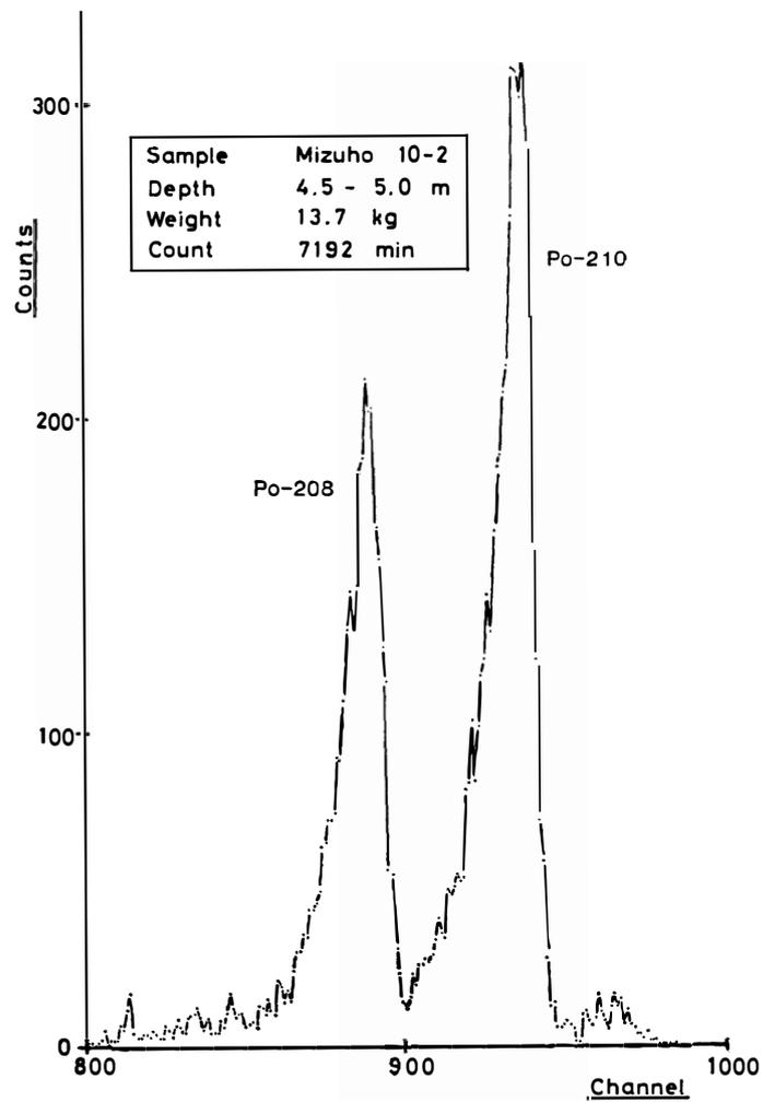
Fig. 3. Alpha-spectrum of Po-208 and Po-210.
