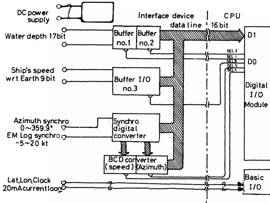
Fig. 1. Block diagram of the interfacing device that receives the navigational signals and converts them to a form acceptable for the CPU unit.
