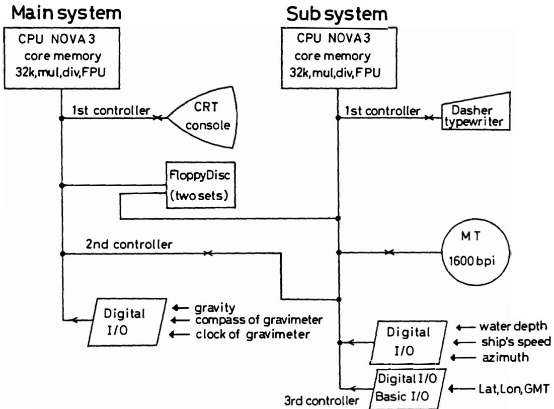
Fig. 2. Interconnections between the units of the computer system.
