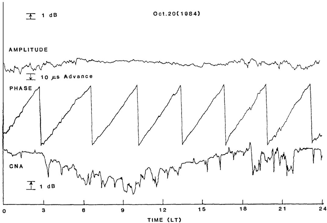
Fig. 3. Example of the data observed by VLF phase tracking receiver and riometer at Tjörnes.
