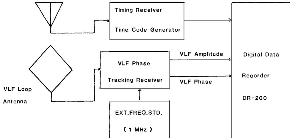
Fig. 1. Simplified diagram of VLF phase tracking receiver system.
