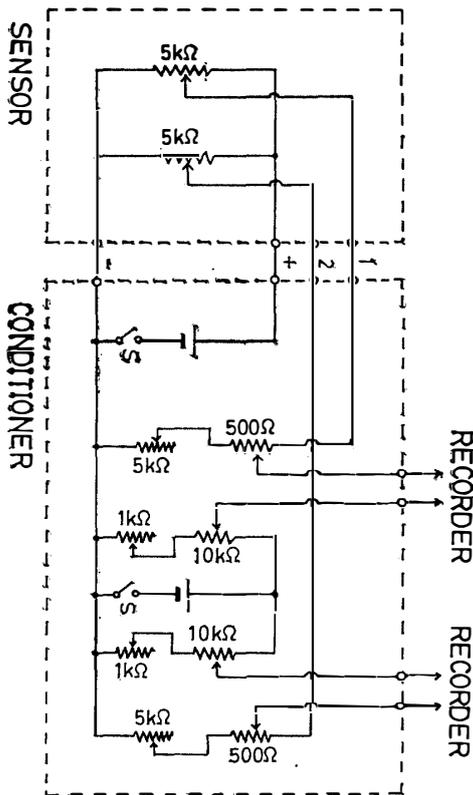
Fig. 3. Schematic diagram of the circuit of measurement system.
