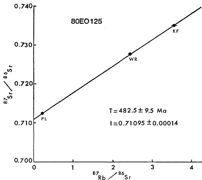
Fig. 2. Rb-Sr mineral isochron plot for granitic gneiss from Syowa Station.
