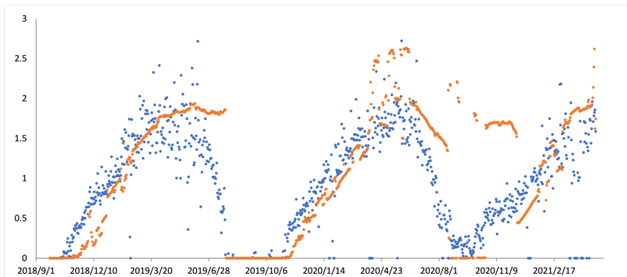
Fig 1. Time-series of the ice thickness observed by moored Upward Looking Sonar (blue dots) and accumulated ice-thickness (orange dots) in the Beaufort Sea
