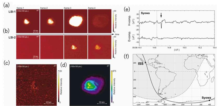
Figure 4. (a) Lightning and sprite images measured by the GIMS wideband camera (LSI-1) and narrowband camera (LSI-2). (b) Results of the image subtraction between LSI-1 and LSI-2. (c), (d) Results of the image subtraction between LSI-1 and LSI-2. Dot structures corresponding to sprite emissions can be confirmed in Figure 4(d). (e), (f) ELF waves excited by the sprite-producing lightning discharges.
