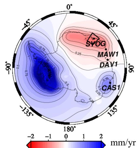
Figure 2. Spatial distribution of the estimated vertical elastic deformation rate due to recent snow mass change. The snow mass change is estimated from GRACE.
