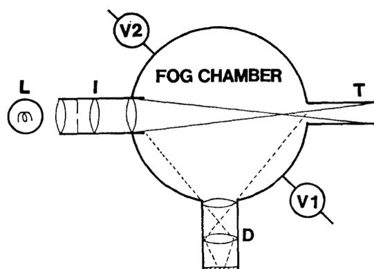
Fig. 1. Optical system of the fog chamber (top view). L, halogen lamp; I, illuminator; D, photodetector; T, light trap.
