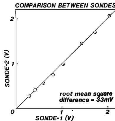
Fig. 4. Comparison between two identical fog chambers.
