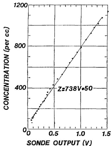
Fig. 3. Relation between DC output of fog chamber (volt) and concentration measured with Pollak counter ( $\text{cm}^{-3}$ ).
