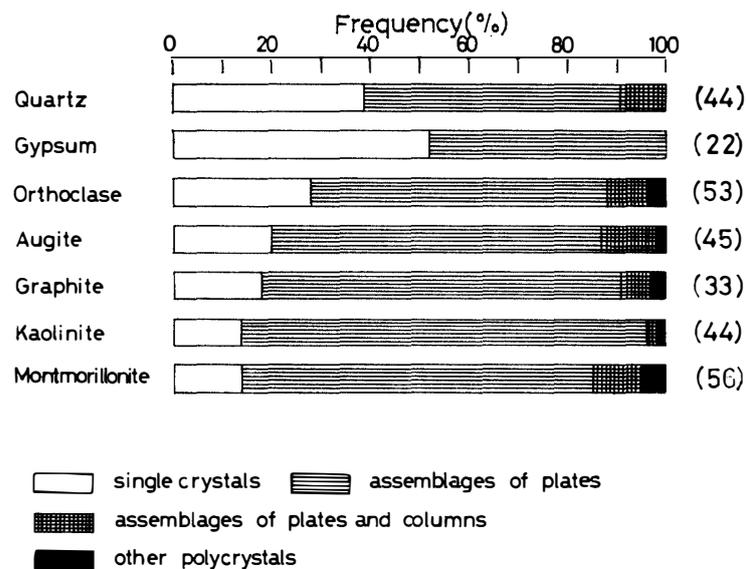
Fig. 3. Frequency of ice crystals of each type when seeded with seven kinds of ice nuclei. Numerals in parentheses show the number of observed crystals.
