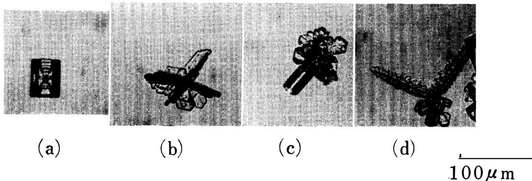
Fig. 2. Ice crystals grown at temperatures about  $-25^{\circ}\text{C}$ . (a) Column, quartz, (b) Assemblage of plates, quartz, (c) Assemblage of plates and columns, orthoclase, (d) Peculiar shape, orthoclase.
