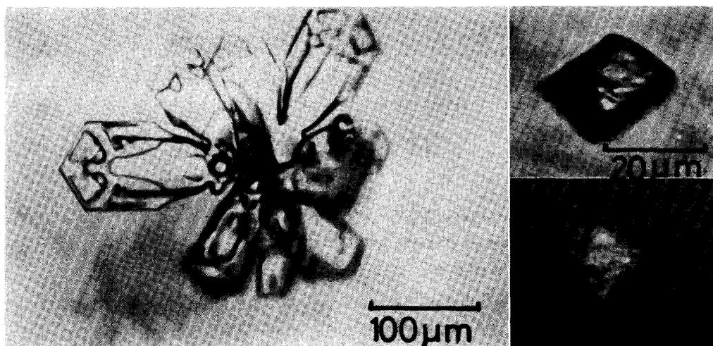
Fig. 5. An ice crystal of polycrystalline type and its nucleus (in transmitted light and in transmitted polarized light).
