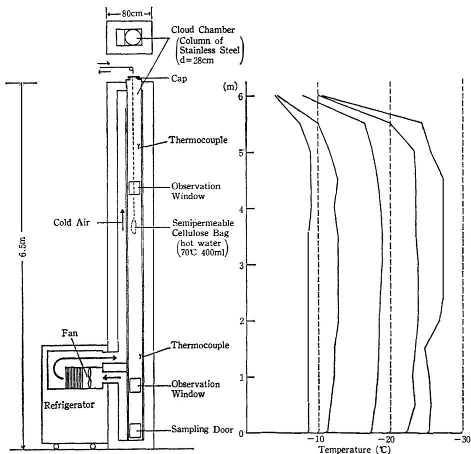
Fig. 1. Large cloud chamber and vertical temperature profiles in the chamber.
