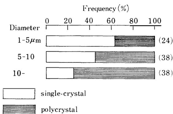
Fig. 4. Frequency of ice crystals of single-crystalline and polycrystalline types. Ice crystals were produced by seeding orthoclase at temperatures about  $-15^{\circ}\text{C}$ .
