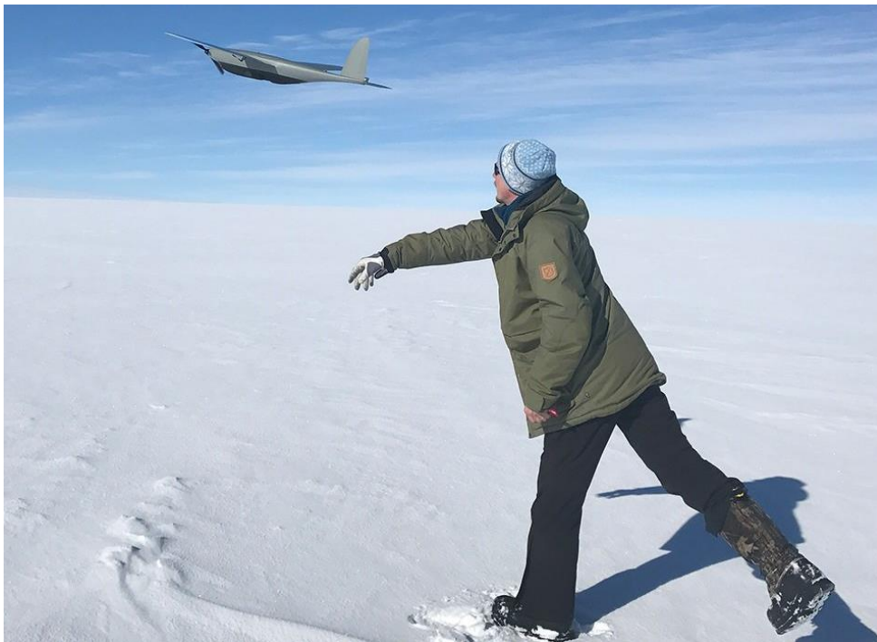
Figure 1. Aslak Grinsted launching the Cumulus one fixed wing drone. The drone collect a set of photos that are used to create an elevation model and a georeferenced ortho-photo. Repeat mapping will allow us to measure displacement using optical feature tracking providing high-resolution ice velocities.
