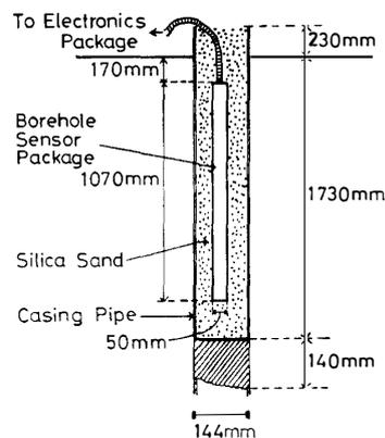
Fig. 2. A schematic view of the installation of the borehole type tiltmeter.
