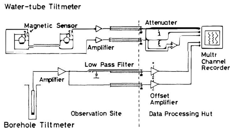
Fig. 3. Block diagram of the ground tilt observation. The borehole type and the water-tube tiltmeters are shown. The details of the water-tube tiltmeter are described by KAMINUMA and NAGAO (1983).
