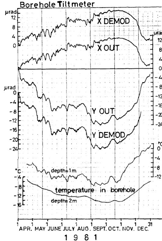
Fig. 4. Ground tilt of four output signals of the borehole type tiltmeter and underground temperature at 1 m and 2 m depths at Syowa Station.
