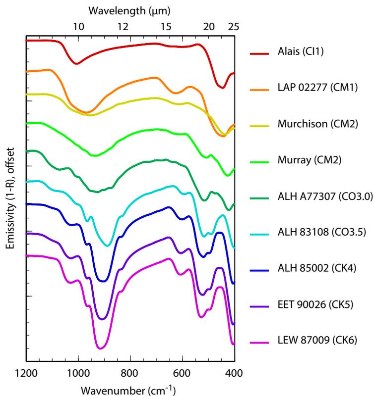
Figure 1. TIR spectra of carbonaceous chondrites ranging from petrologic type 1 – 6 showing the range from aqueous alteration (phyllosilicate-dominated) to thermal metamorphism (olivine-dominated).
